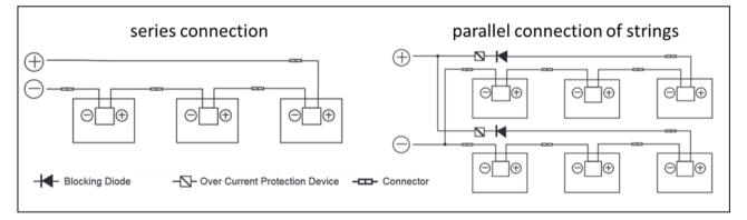
Suitable overcurrent protection measures (e.g. string cut-out) are required for the parallel connection of the modules. It must be ensured that the specified capacity regarding the return current IR of the datasheet will not be exceeded. If there are more than two parallel strings, string fuses and string diodes must be used.
