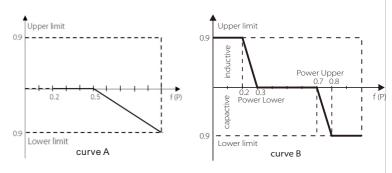
Reactive power control, Reactive standard curve Q = f(V)
