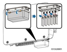
Figure 5-4 Removing the AC terminal box
