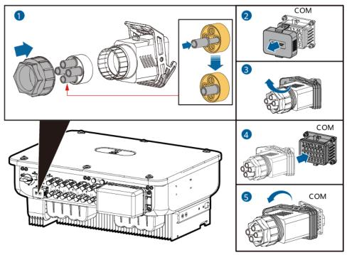
Figure 5-13 Securing the signal cable connector
