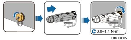
• WLAN-FE Smart Dongle (FE Communication)
