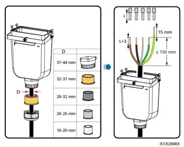
Figure 5-5 Stripping the AC power cable
