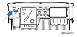
Figure 4-13 Installing the locking screw for the DC switch
