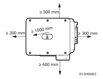
• When installing multiple SUN2000s, install them in horizontal mode if ample space is available and install them in triangle mode if no ample space is available. Stacked installation is not recommended.
