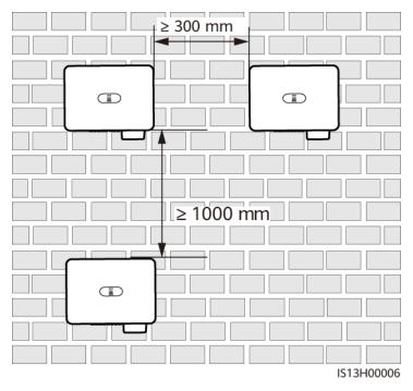
Figure 4-6 Stacked installation (not recommended)
