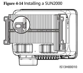
Step 3 Tighten the nuts on both sides of the SUN2000.
