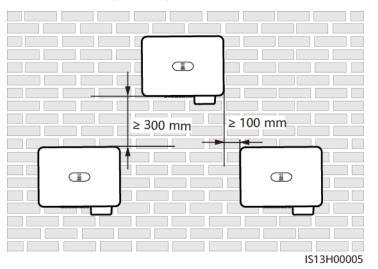
Figure 4-4 Two-layer triangle installation (recommended)
