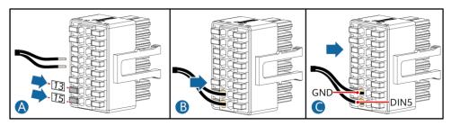
2. Connect the signal cable connector to the communications port.
