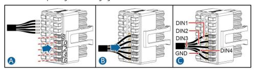
• Connect the rapid shutdown signal cable.
