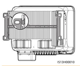
3. Tighten the security Torx screws on both sides.
