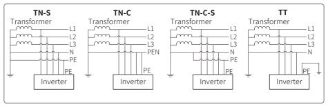
Note: For TT grid structure, RMS voltage between neutral wire and earth wire must be less than 20V.
