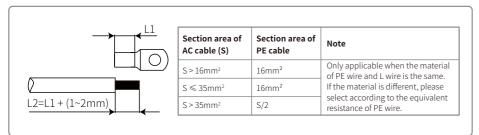
2. Insert the stripped wire into the terminal and compress it tightly by crimping pliers.
