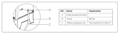
4. In order to improve the corrosion resistance of the terminal, it is recommended to apply silica gel on the earth terminal for corrosion protection after the grounding cable assembly is completed.
