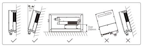
To ensure heat dissipation and convenient disassembly, the minimum clearance around the inverter should not be less than the following values.
