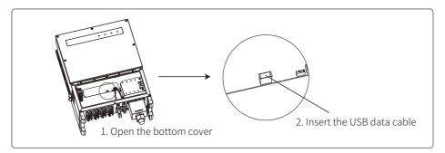
This function is only for local firmware upgrade and parameter calibration.
