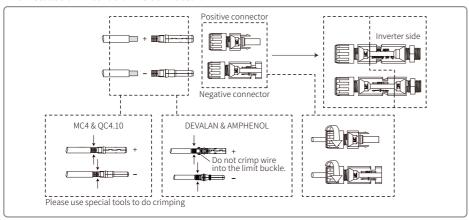
In order to better dustproof and waterproof the internal inverter, all the DC connectors provided by accessory bag should be connected to the inverter. If only some of the DC connectors are used, the DC connectors without connection should be blocked with non-conductive insulator.
