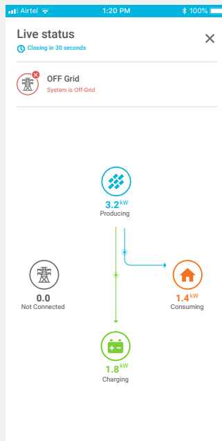
Solar production is powering the home and charging the batteries.
