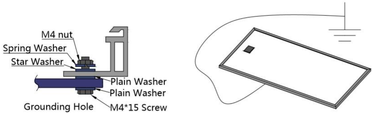
Figure 10: Ground installation of PV modules
