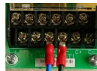
Figure3.3.3-5 (Remove the short wire)
