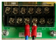
Figure3.3.3-2 (B+ and B- are reversed)
