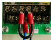
Figure3.3.3-3 (Connect the corresponding position with a short wire)
