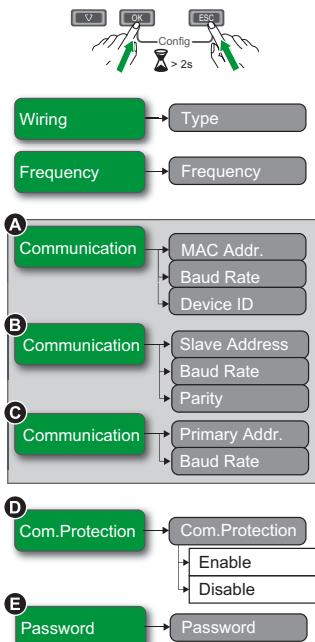
**en** Enter configuration mode and configure basic metering, communications, and security settings (see section 7 for instructions)
