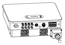
Figure 4-8 Removing AC waterproof cover diagram
