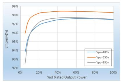
Figure 2-9 Power efficiency curve (take 20KW for example)
