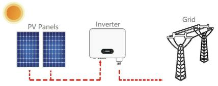
Figure 2-1 PV Grid-Tied System
