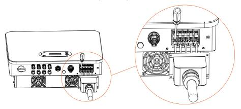
Figure 4-10 AC cable connection instruction diagram (2)
