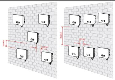
Figure 3-3 Clearance for multiple inverters
