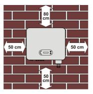
Figure 3-2Clearance for single inverter
