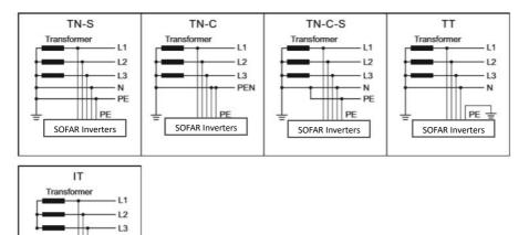
Figure 2-2 Overview of the grid configurations
