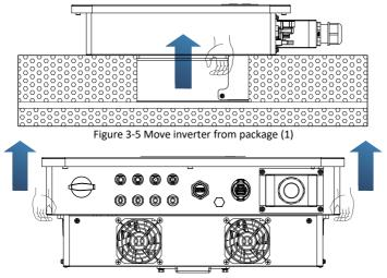
Figure 3-6 Move inverter from package (2)
