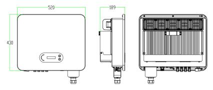
Figure 2-3 Front, side and back of the machine (15~24K)
