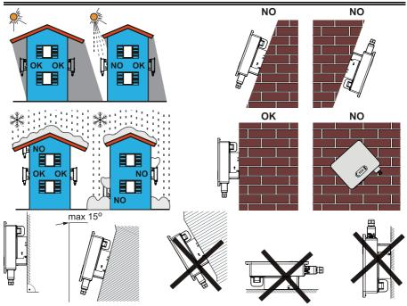
Figure 3-1Installation Position Selection
