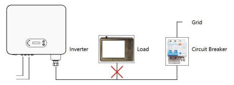
Figure 4-5 Incorrect connection between load and inverter
