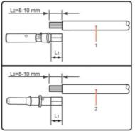
Figure 4-11 DC cable connection (1)
