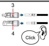
Figure 4-13 DC cable connection(3)
