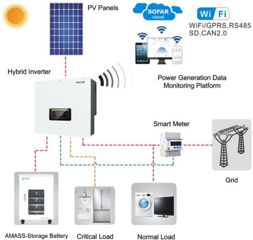
Fig. 3-1 Typical Energy Storage System
