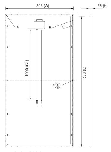
A: 4 x drainage 10\*10 mm B: 16 x ventilation hole 3\*7 mm
