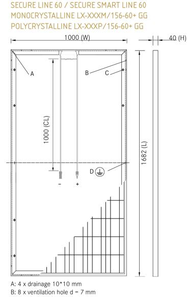
C: 8 x mounting hole  $d = 7 \text{ mm}^{**}$
