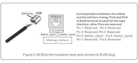
3. Connect RJ45 to DRM (logic interface).
