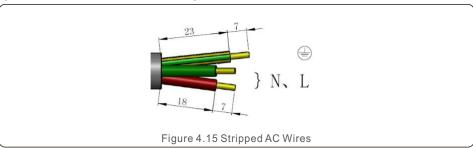
b) Fix the wires into the correct postion. Torque 0.8N.m
