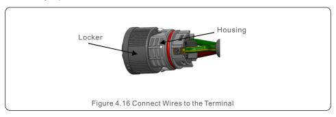
c) Insert Seal and Clamp Finger into body ,then tighten the nut, torque 2.5+/-0.5N·m.
