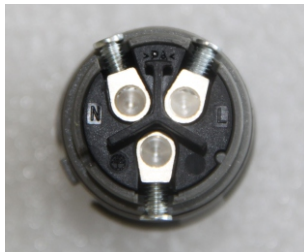
▲ Figure 4.13 AC Grid Terminal Connector Inside
