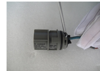
▲ Figure 4.16 Connect Wires to the Terminal
