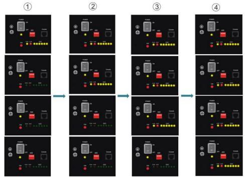
If all the battery LED lights on, and then off, which means the battery system is good and working.
