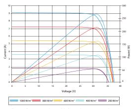
Excellent performance under weak light conditions: at an irradiation intensity of 200 W/m² (AM 1.5, 25 °C), **96.5%** or higher of the STC efficiency
