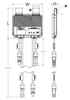
\*Clips can be removed for rack mounting
