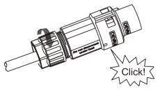
Push the threaded sleeve to connection terminal until both are locked tightly on the inverter.
