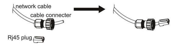
Step 4: Insert the cable connector into COM port at the bottom of inverter and screw it tightly. Then insert other side of the network cable into PC or other device.
