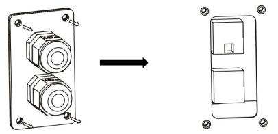
Step 2: Prepare a standard network cable and cable connector, then insert the network cable through the cable connector.
