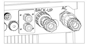
• Loosen the cap on the terminal, pull the threaded sleeve out of the socket.
