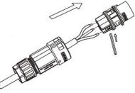
Push the threaded sleeve into the socket, tighten up the cap on the terminal.
