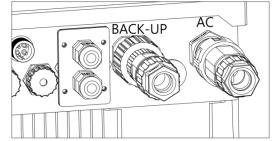
• Remove the AC connector: Press the bayonet out of the slot with a small screwdriver or the unlock tool and pull it out, or unscrew the threaded sleeve, then pull it out.
