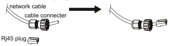
Step 3: Insert the cable connector into BMS port at the bottom of inverter and screw it tightly.
