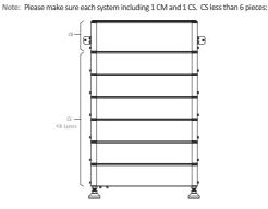
Place the battery 20mm against the wall. Note: Please make sure the Operating Status LED is on your left handside when you facing the battery model.
