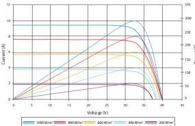
Excellent performance under weak light conditions: at an irradiation intensity of 200 W/m<sup>2</sup> (AM 1.5, 25 °C), **96.5%** efficiency (200 W/m<sup>2</sup>) is
