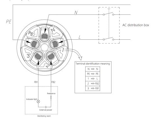
Step 3: Tighten wires as shown in the figure below. Tightening torque 0.6±0.1N·m, then insert cable respectively to pin hole.
