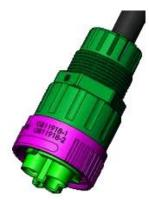
Step 5: Insert seal into body, then tighten the nut, torque  $1.5\pm0.3$ N·m. The maximum spacing between the nut and the body after tightening is 1.5mm.
