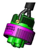
Step 4: Screw body to housing, tightening torque 1.2±0.2N·m.
