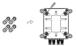
• Choose the place you want to install the S-BOX. Place the S-BOX on the wall and mark the position of the 4 holes from fixing blocks.
