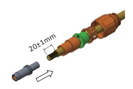
4. Clamp the terminal with a hydraulic clamp.
