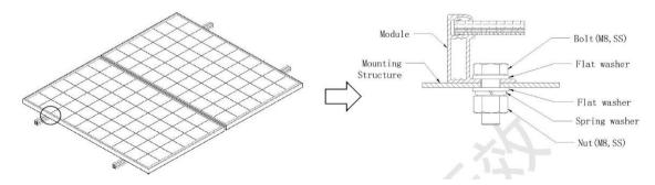
Figure 3 Mounting holes
