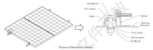
Figure 4 Mounting clamps
