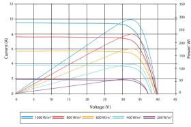
Excellent performance under weak light conditions: at an irradiation intensity of 200 W/m<sup>2</sup> (AM 1.5, 25 °C), **98**% efficiency (200 W/m<sup>2</sup>) is achieved
